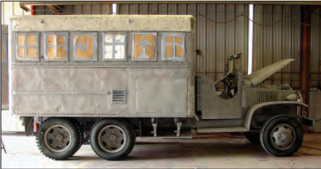
The GMC CCKW shop van was completely sandblasted and primed at a local shop in Waller, Texas.
