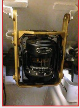
This hard to find item is a directional compass assembly, with mount made by Sherrill Research Corporation Model AEG-1 Mfg. 1944. The compass allowed the assistant driver to know the direction they were traveling and helped orient him to a map grid reference while buttoned up under combat conditions.
