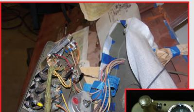
The instrument panel and wiring harness was tested over and over before it was reinstalled. We used a portion of an NOS harness and wanted it to be totally functional.
