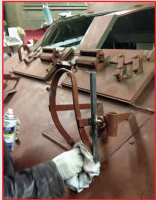
The metal flag mounts were reproduced to the exact size based on the Photoshop images superimposed over the M20.
