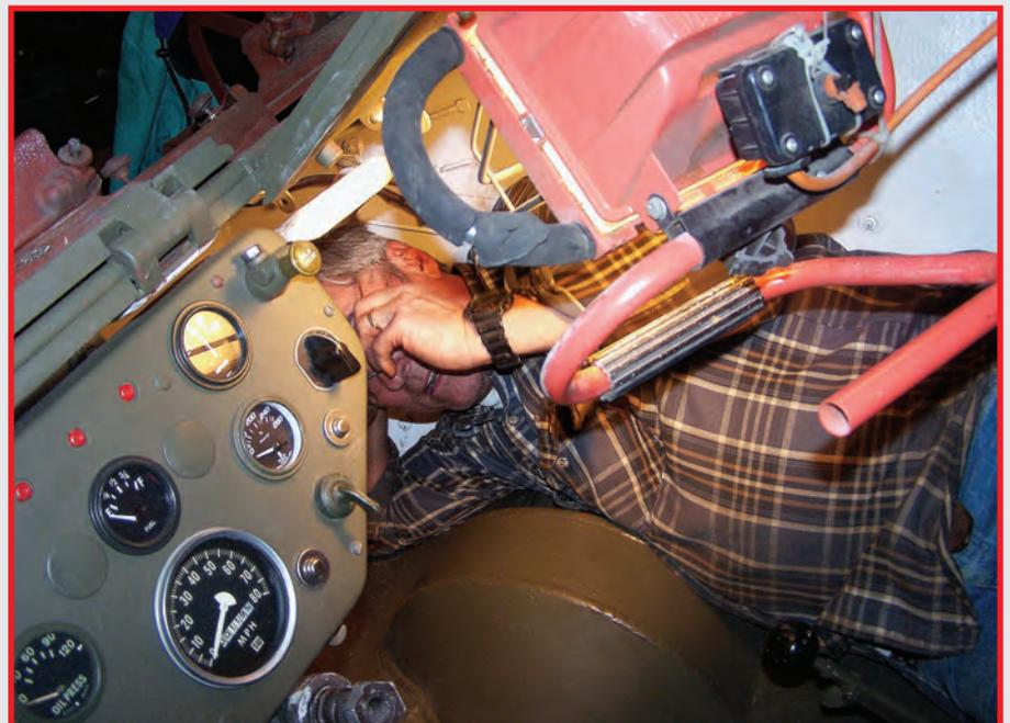
Denny Hair examines the wiring harness connections in a tight space. Getting stuck in the M20 happened frequently during the restoration because the vehicle was designed for a smaller generation of men.
