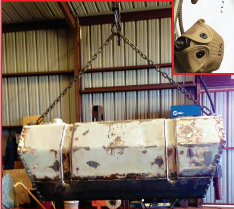
The metal gas tank shroud that housed the bladder was reworked. The gas line was run from underneath into the stainless steel tank. We use aviation fuel to keep the fuel pump seals from deteriorating.
