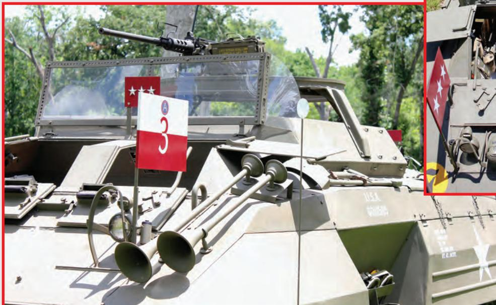
The restored M20 – driver's side front. It is complete with all of the tools, markings and air horns, now replicated as it was in 1944.
