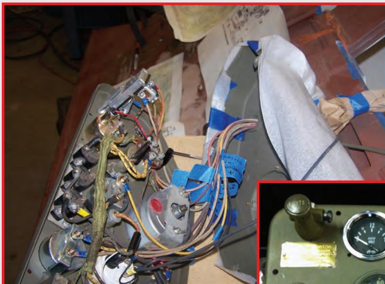
The instrument panel and wiring harness was tested over and over before it was reinstalled. We used a portion of an NOS harness and wanted it to be totally functional.
