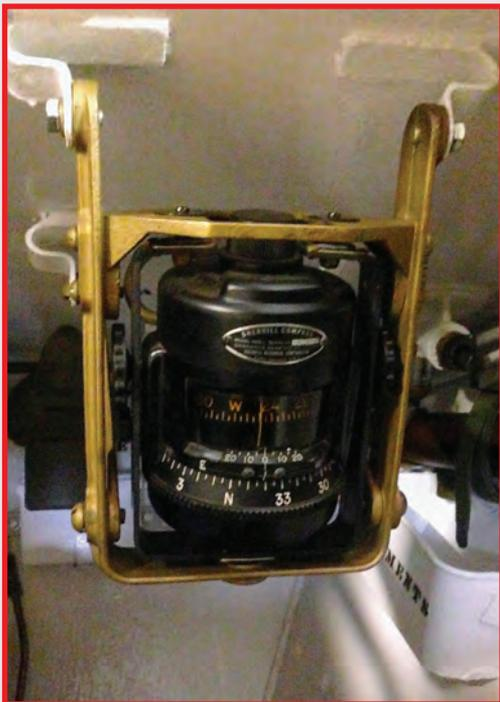
This hard to find item is a directional compass assembly, with mount made by Sherrill Research Corporation Model AEG-1 Mfg. 1944. The compass allowed the assistant driver to know the direction they were traveling and helped orient him to a map grid reference while buttoned up under combat conditions.
