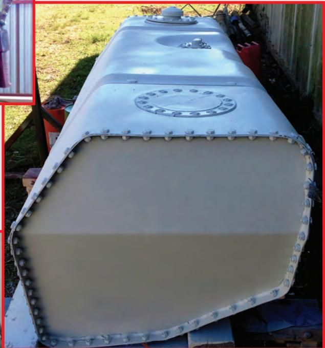
The original bladder was installed by removing all the bolts from one end. We designed a 25-gallon, custom-made stainless steel tank (approximately half the capacity of the bladder) and mounted it in the shroud. Modern fuels would likely dissolve an original bladder and clog the fuel system.
