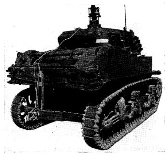
FIGURE 2.—Rear view of motor carriage M8, showing quick release hitch for trailer.
