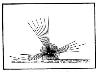
FIGURE 25.—Ricochet burst.
