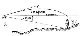
FIGURE 38.—Angle of site and its effect on the trajectory.
