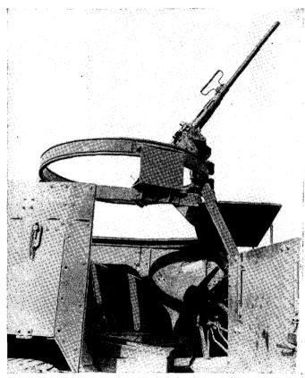
FIGURE 8.—Caliber .50 machine gun on ring mount.
