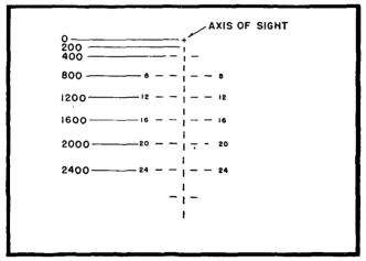
FIGURE 21.—Reticle, coaxial telescope, with dimensions.
