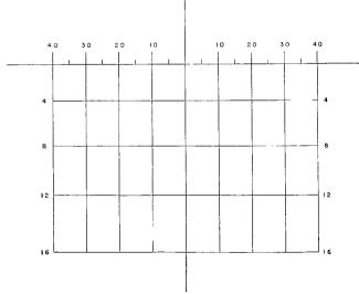
FIGURE 15.—Reticle, panoramic telescope M12A5.
