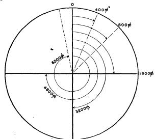
FIGURE 32.—Measuring angles in mils,
