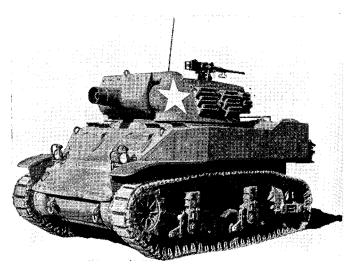
FIGURE 1.—75-mm assault howitzer on motor carriage M8.
