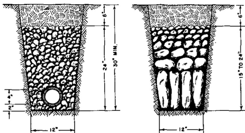
FIGURE 4.—Tile and stone subdrains.
