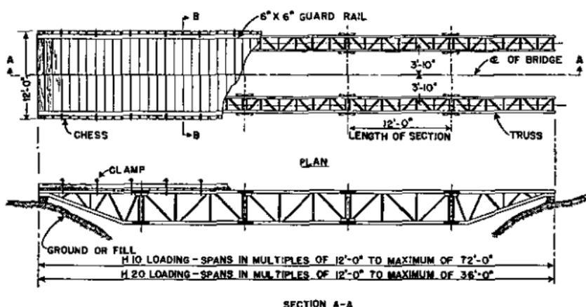
FIGURE 59.—Portable single span for division loads (H-10).
