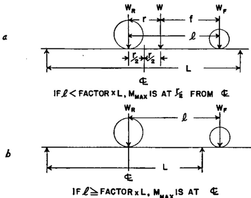
FIGURE 32.—Positions of heavier axle load on bridge to produce maximum bending.
