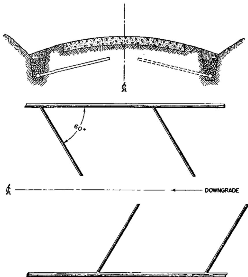
FIGURE 5.—Method of employing lateral drains.
