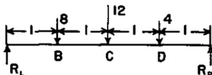
FIGURE 31.—Simple beam with three unequal loads.
