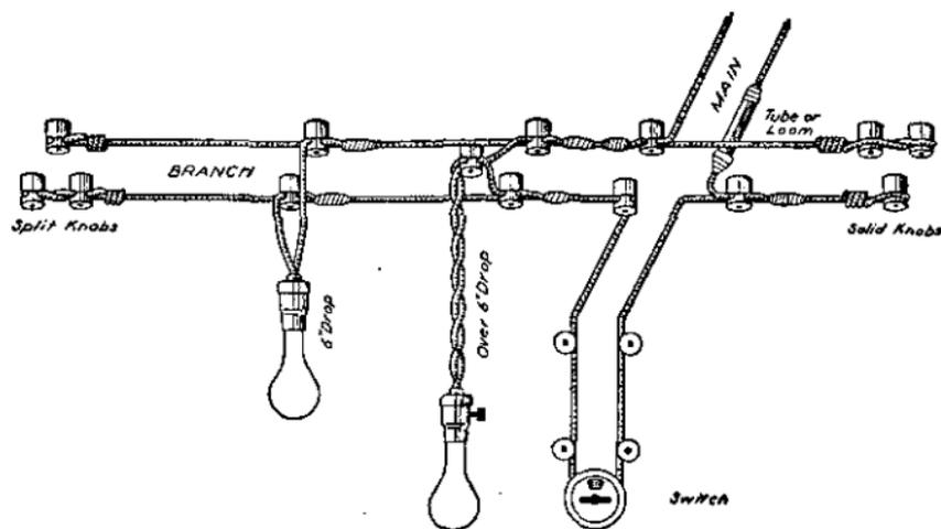
FIGURE 129.—Lighting installation using porcelain knobs.
