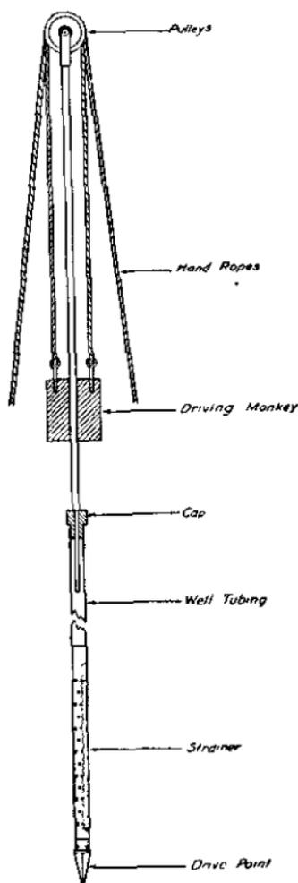
FIGURE 125.—Construction of driven well.
