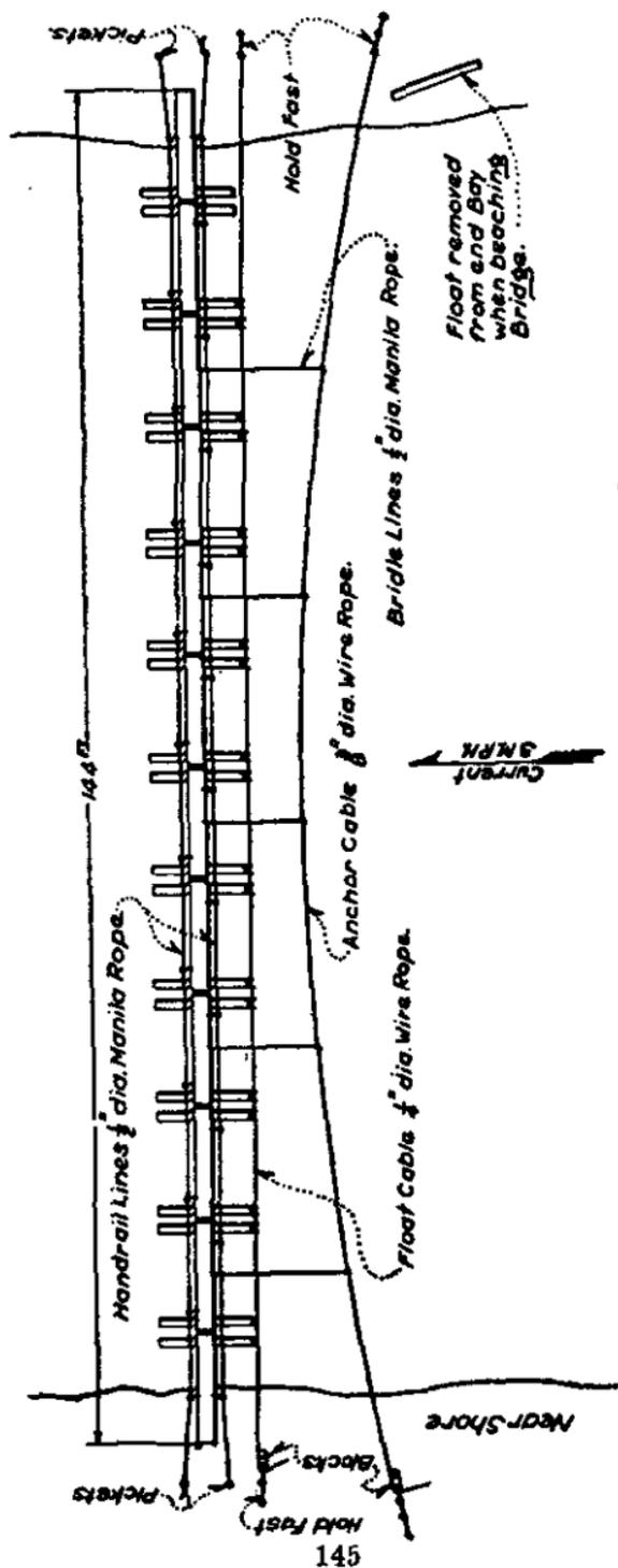
FIGURE 43.—Assembled footbridge using anchor and float cables.
