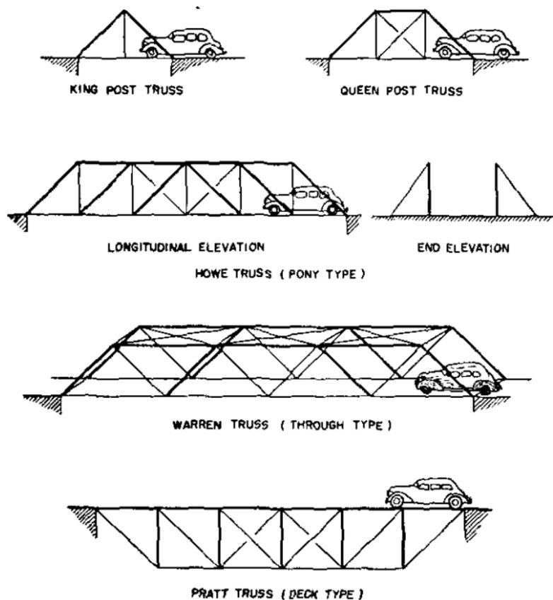
FIGURE 38.—Types of trusses.
