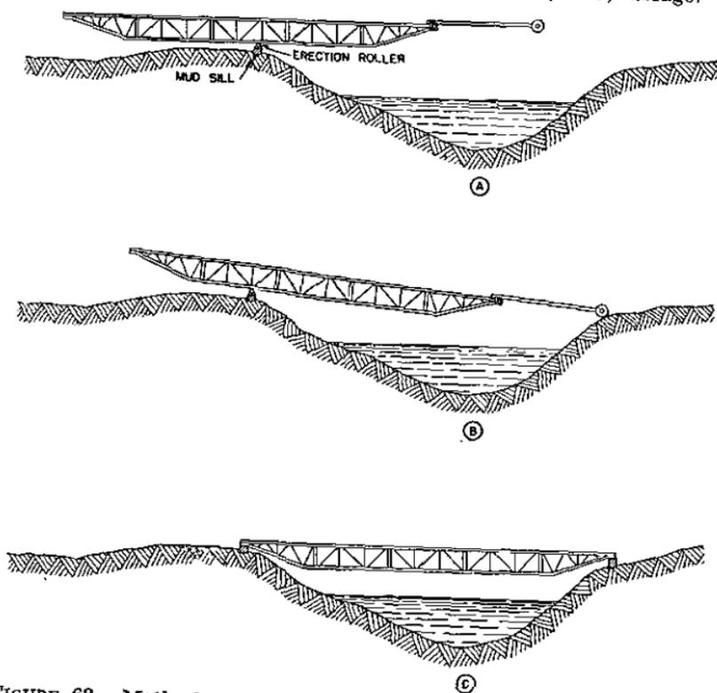
FIGURE 62.—Method of launching and installation on abutments.
