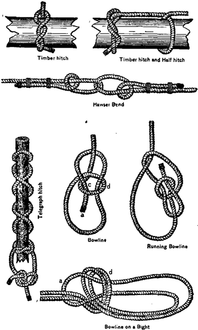
FIGURE 140.—Types of knots—hitches, bends, and bowlines.
