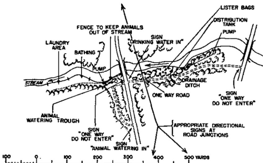
FIGURE 120.—Typical water-distributing point.
