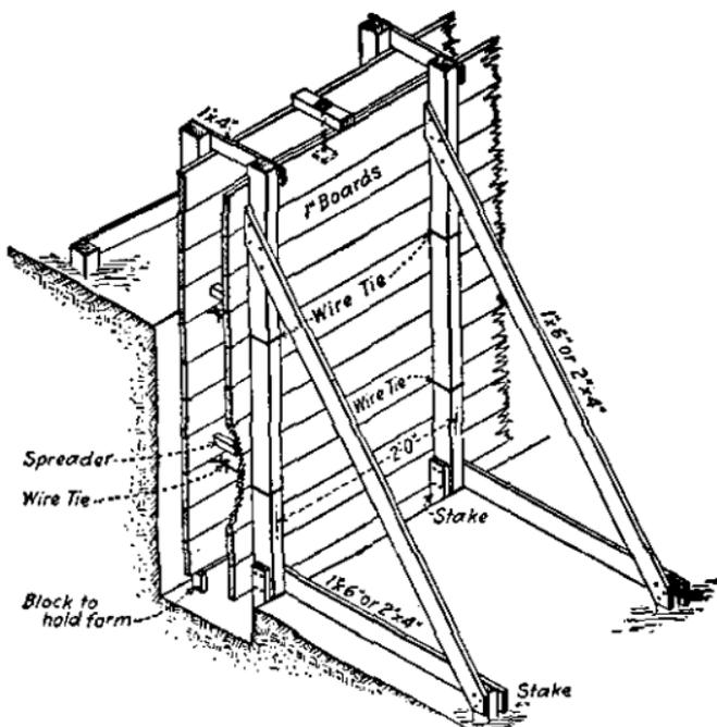
FIGURE 151.—Typical externally braced form.
