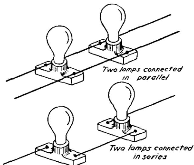
FIGURE 130.—Comparison of parallel and series circuits.
