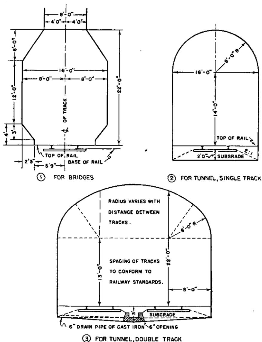
FIGURE 80.—Standard clearance diagrams for bridges and tunnels.
