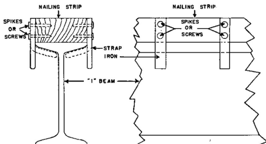
FIGURE 34.—Method of fastening nailing strip to I-beam.
