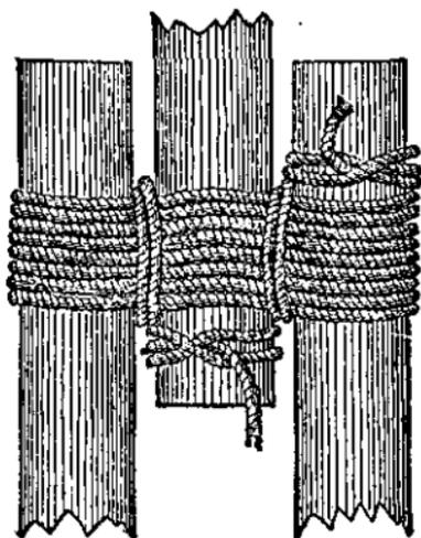
FIGURE 146.—Lashing for tripod.
