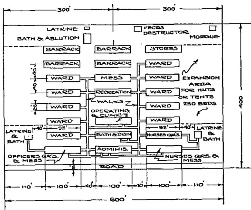
FIGURE 114.—Typical layout for 250-bed station hospital. Individual wards are constructed for normal capacities of 25 and 50 patients. Figure 115 shows the two types of wards. Table LI gives a corresponding bill of materials.
