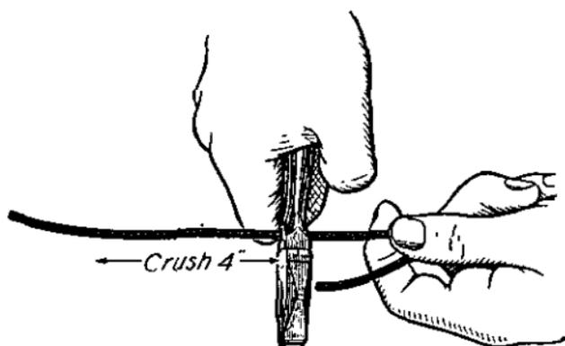
FIGURE 131.—Crushing insulation on long conductor.
