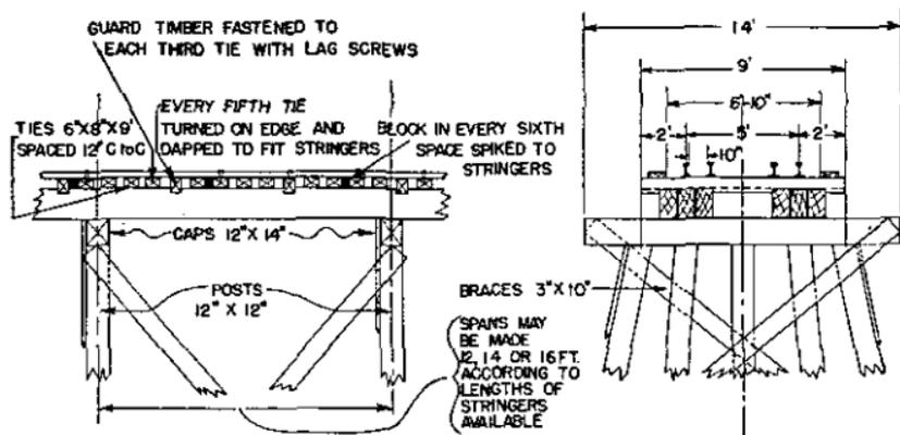
FIGURE 89.—Floor system for standard gage railway timber or pile trestle.
