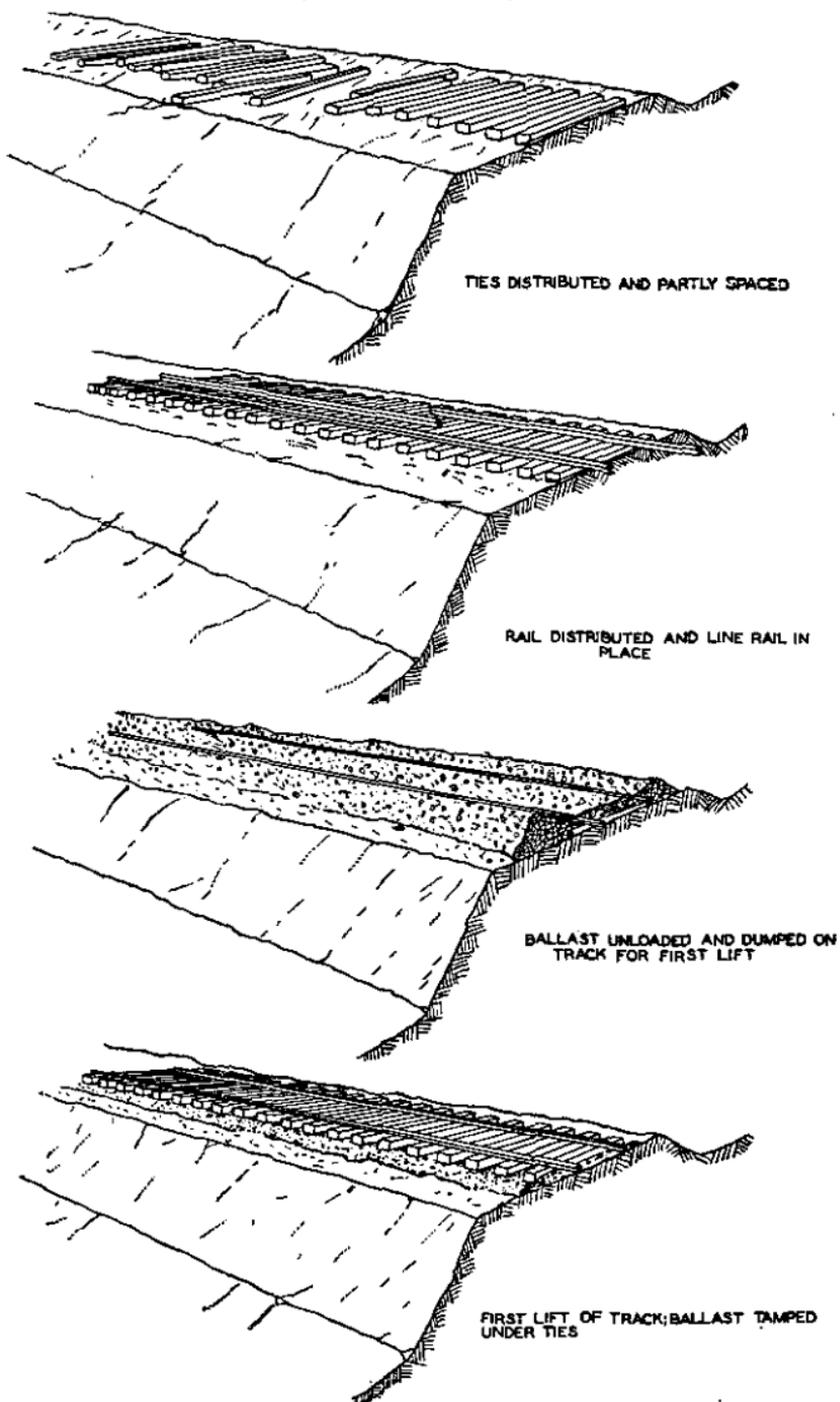
FIGURE 85.—Steps in laying and ballasting tracks.
