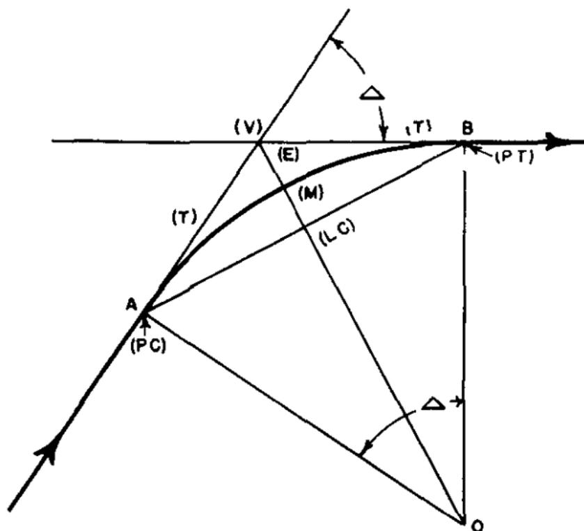
FIGURE 83.—Elements of a curve.
