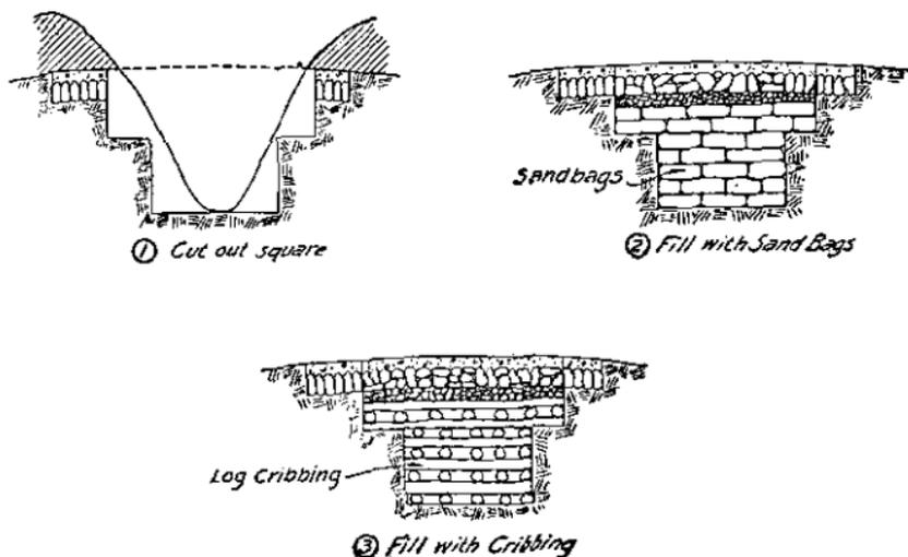
FIGURE 8.—Shell and bomb hole repairs.
