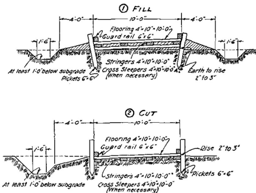
FIGURE 14.—Plank road for motor transportation, fill and cut.
