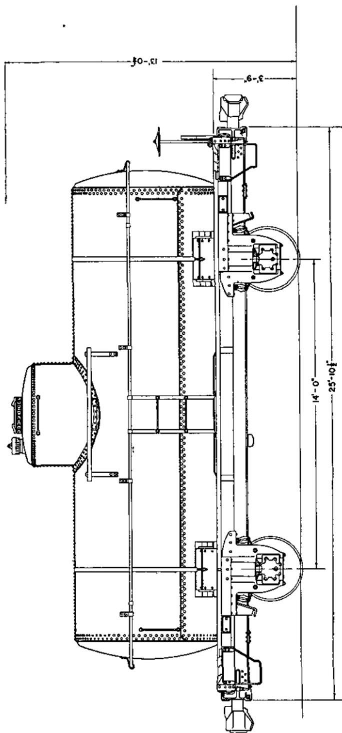
FIGURE 92.—Tank car, 5,000-gallon, 20-ton.
