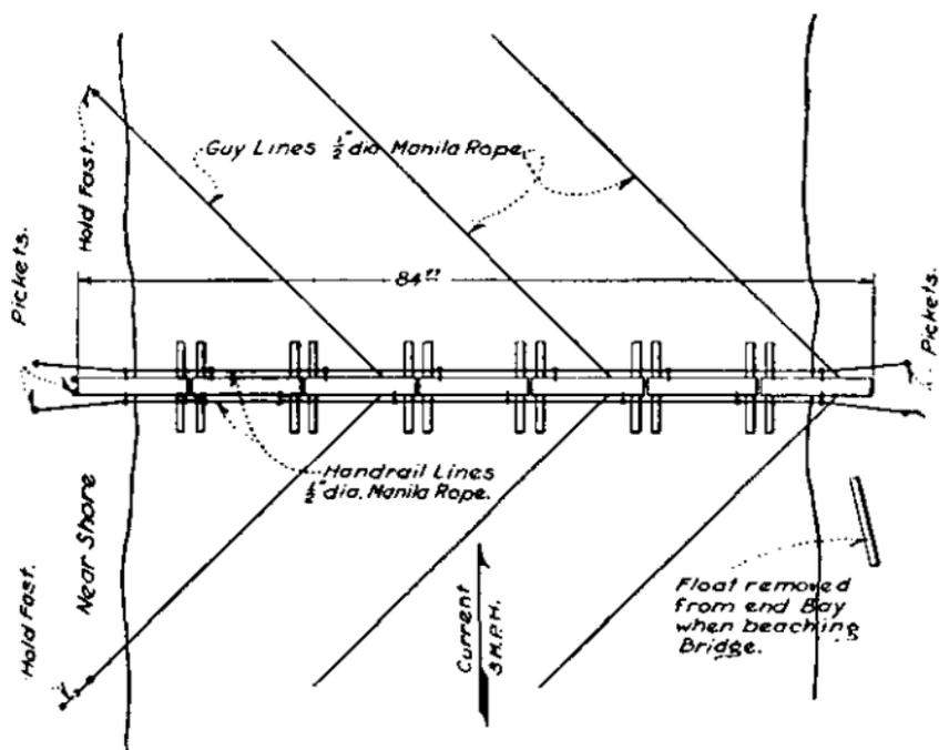
FIGURE 44.—Assembled footbridge using guy lines.
