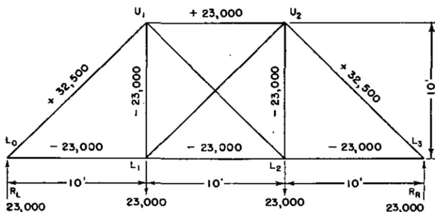
FIGURE 39.—Truss stresses—moments of force.
