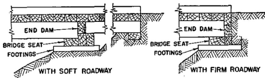
FIGURE 27.—Abutments for simple stringer bridges.
