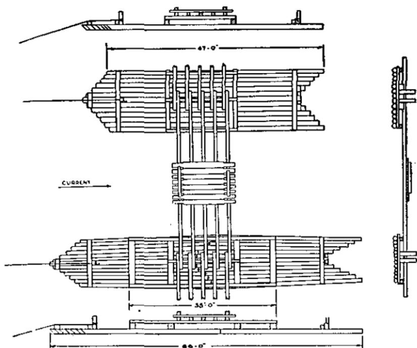
FIGURE 55.—Raft with short and long timber.
