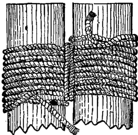
FIGURE 148.—Lashing for shears.
