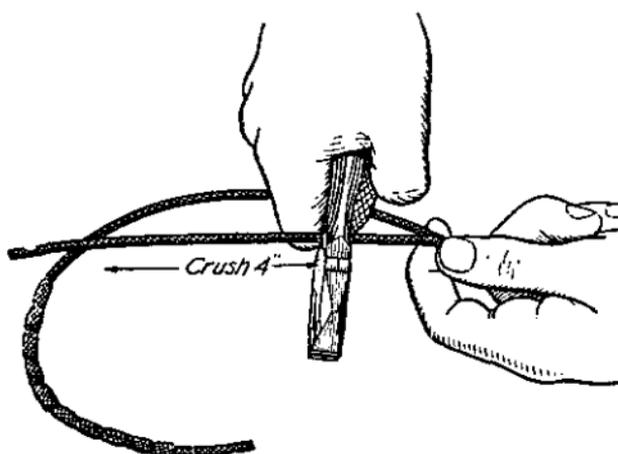
FIGURE 132.—Crushing insulation on short conductor.
