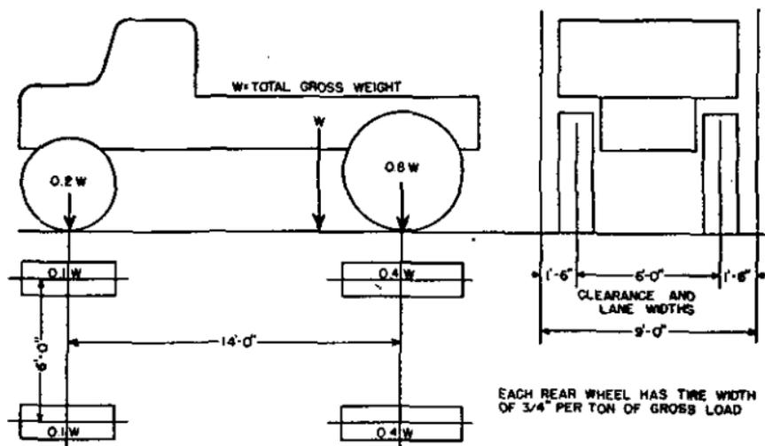
FIGURE 30.—Distribution of wheel loads for design.
