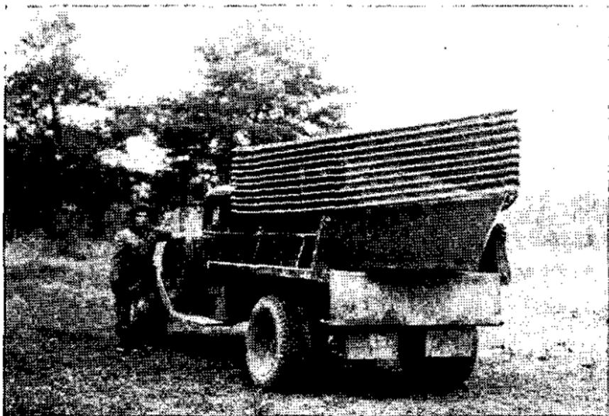
FIGURE 68.—Engineer 1½-ton dump truck with normal load of 10 assault boats.
