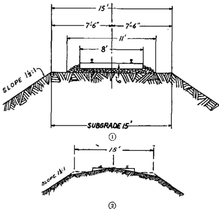
FIGURE 79.—Standard gage roadbed section on embankment.
