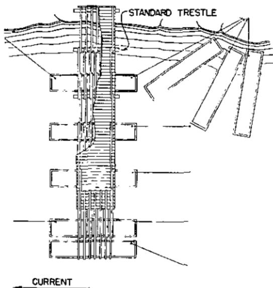
FIGURE 49.—Method of construction by successive pontoons.
