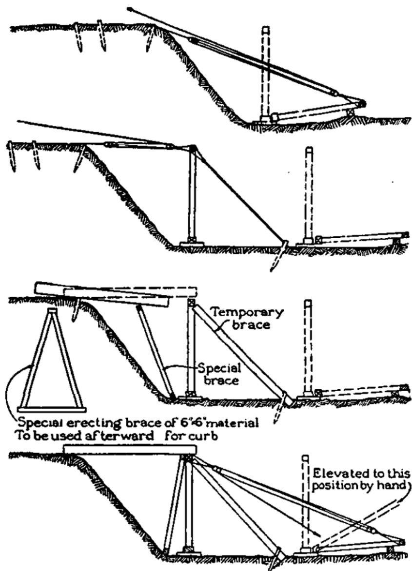
FIGURE 64.—A method of erecting framed trestle bents.
