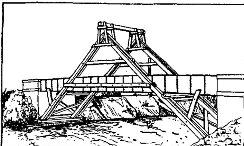
FIGURE 65.—Method of reinforcing girders with A-frame.
