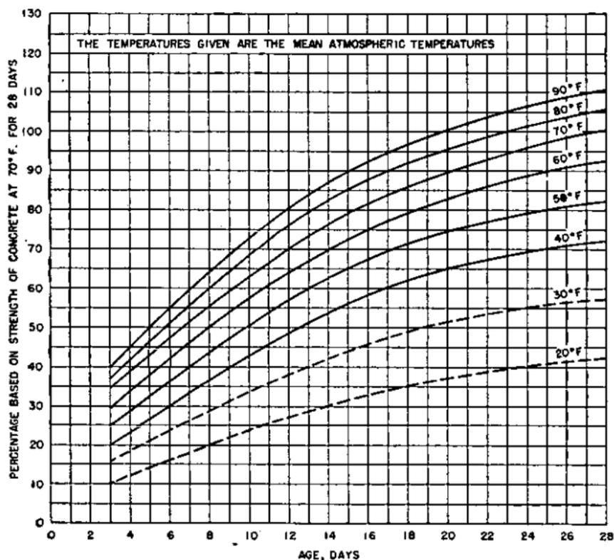
FIGURE 154.—Effect of temperature on strength of concrete.
