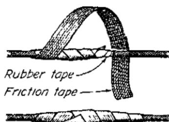
FIGURE 137.—Applying rubber and friction tape.
