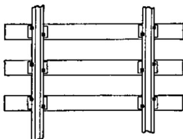
FIGURE 84.—Method of setting spikes.
