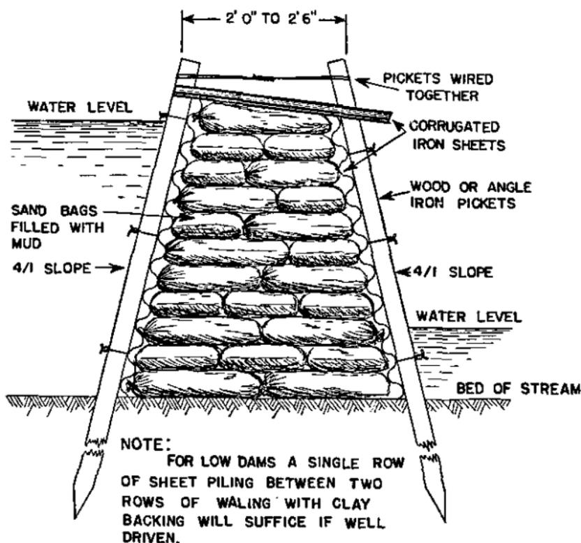
FIGURE 123.—Design for a small dam.
