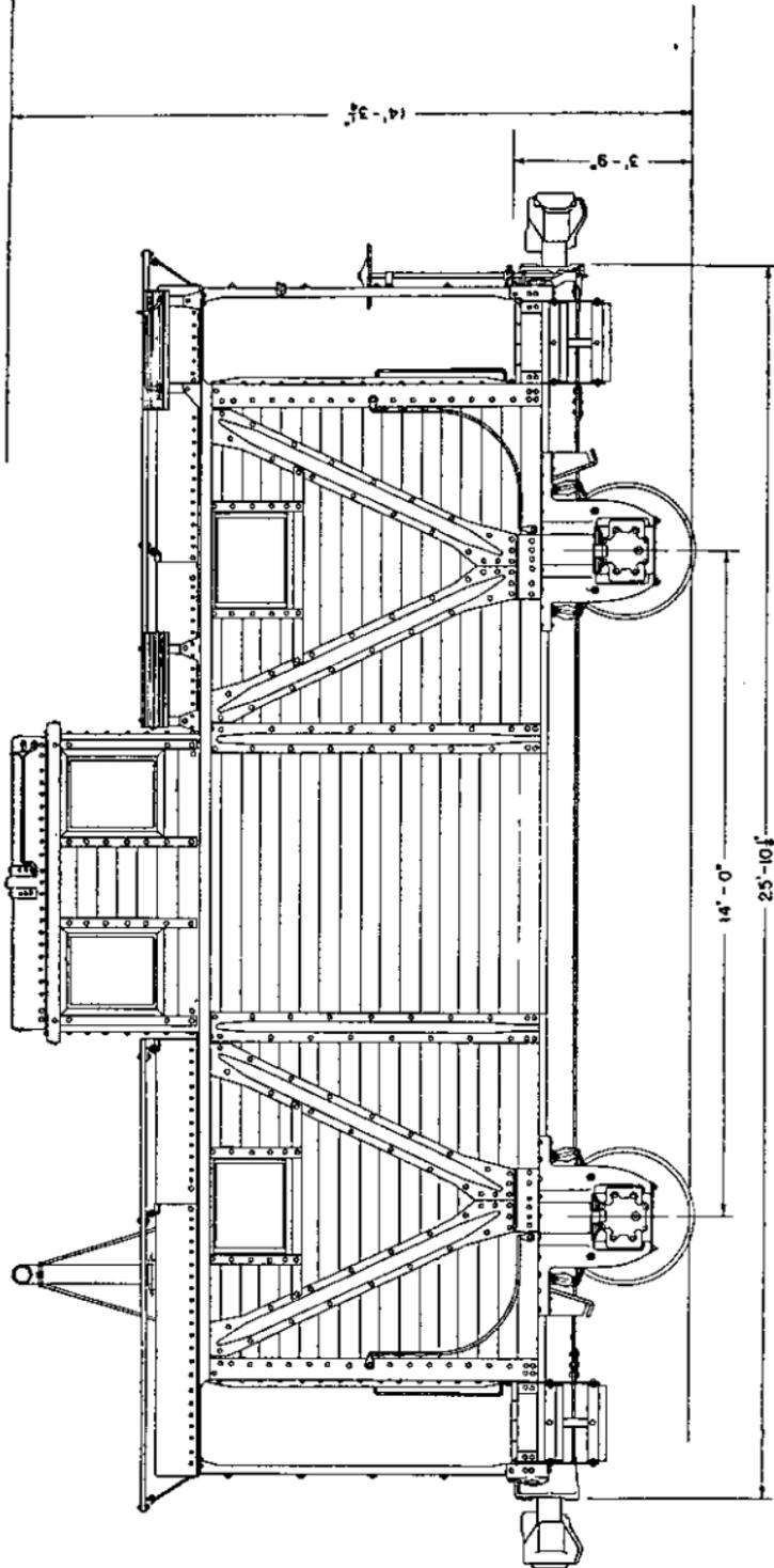
FIGURE 93.—Caboose, 4-wheel, 20-ton.
