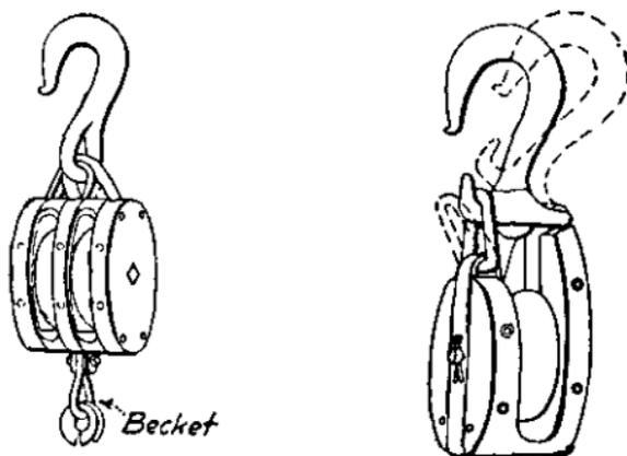
FIGURE 145.—Double wooden block and snatch block.
