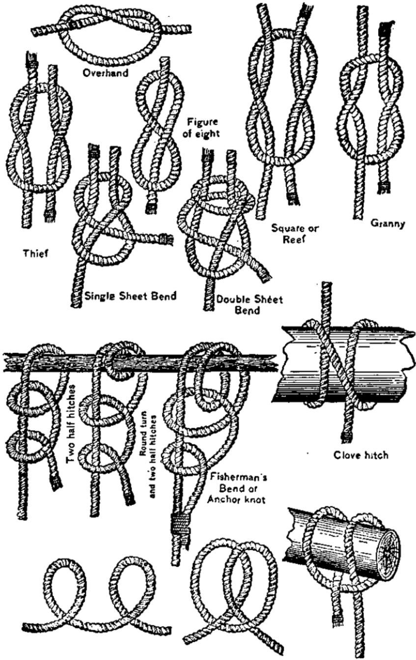
FIGURE 139.—Types of knots—hitches, bends, overhand, etc.
