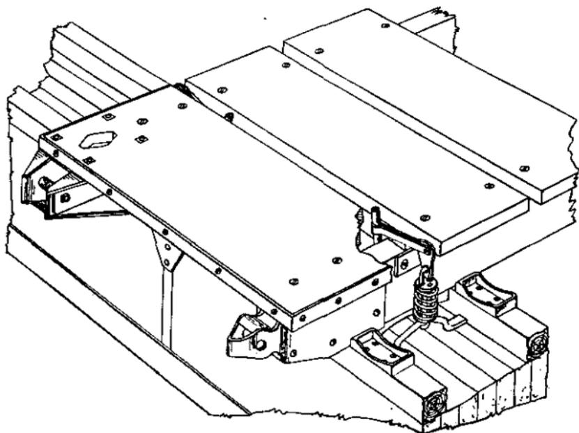
FIGURE 42.—Fasteners between duckboards and floats.
