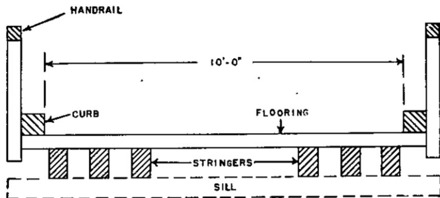
FIGURE 33.—Transverse cross section of typical stringer bridge.
