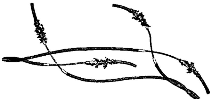
FIGURE 134.—Wires skinned and ready for square knots.
