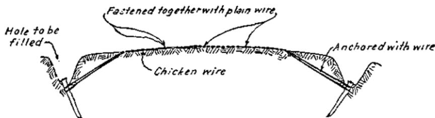
FIGURE 19.—Construction, wire-mesh road.
