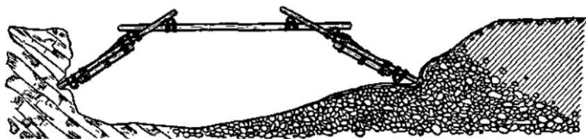
FIGURE 63.—Single- and double-lock spar bridges.
