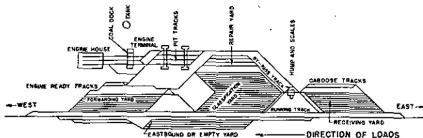
FIGURE 78.—Conventionalized terminal yard layout.
