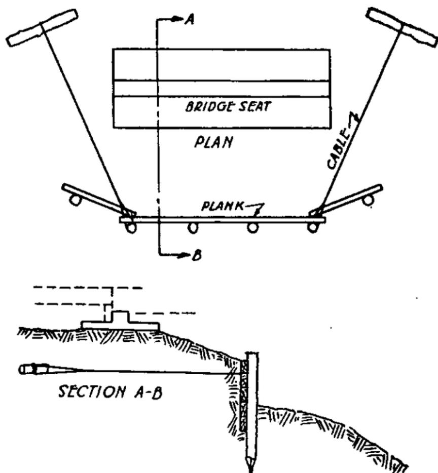
FIGURE 28.—Pile retaining wall.
