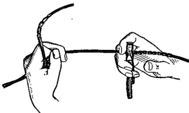
FIGURE 133.—Skinning conductor.
