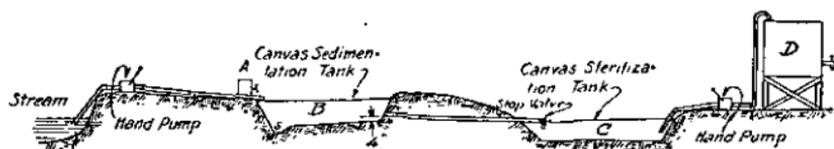
FIGURE 126.—Improvised purification plant.
