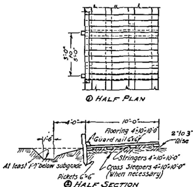
FIGURE 15.—Plank road for motor transportation, plan and section.
