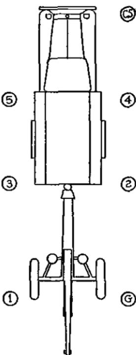
FIGURE 4.—Posts of the cannoneers, carriages coupled.
