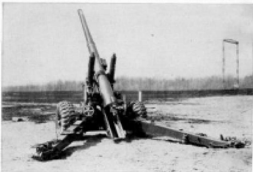
FIGURE 18.—7.2-inch gun on 4.5-inch gun-1.2-inch howitzer carriage (firing position).
