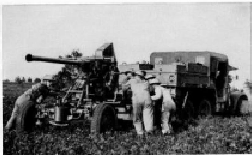
FIGURE 40.—Bofors 40-mm light anti-aircraft gun.
