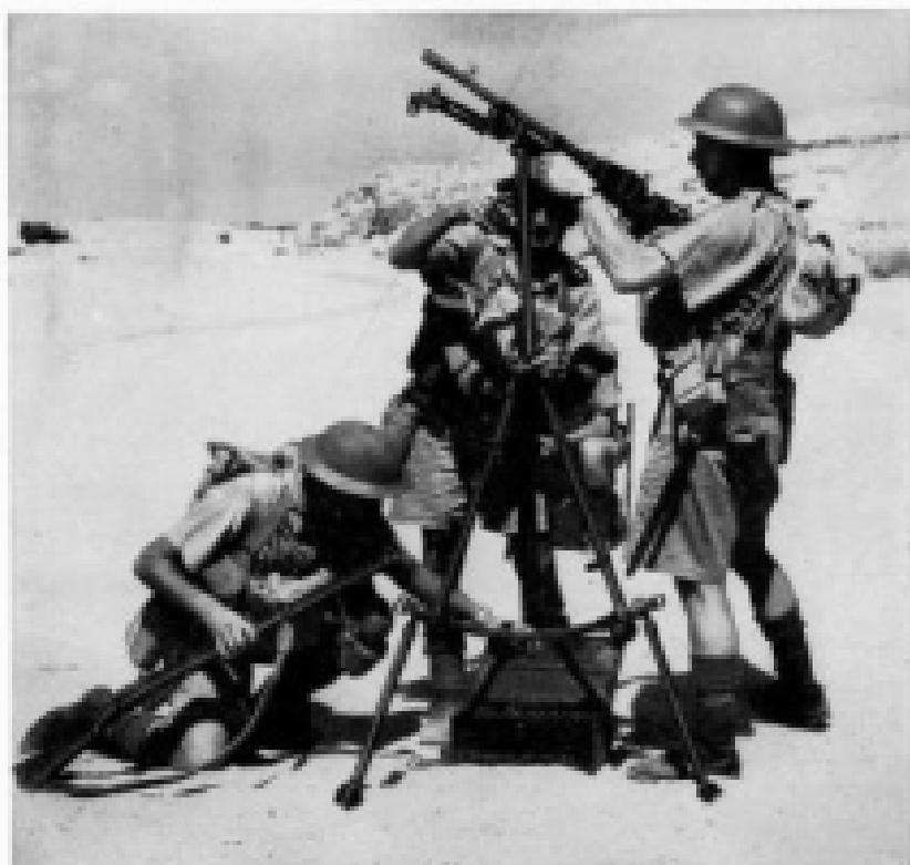
FIGURE 23.—Besa machine gun on anti-aircraft mount.
