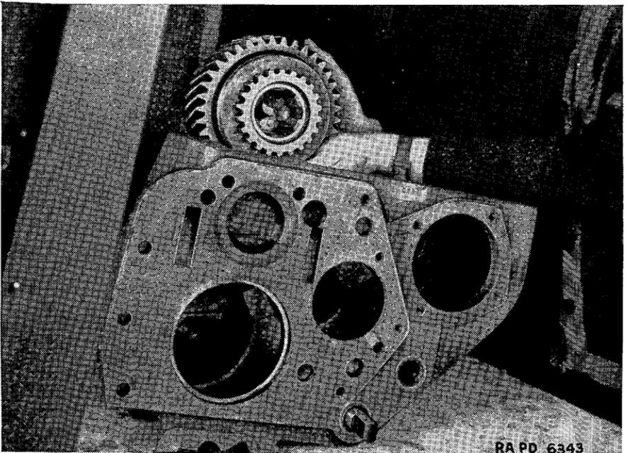
FIGURE 124.—Transfer case mainshaft underdrive gear removal.
