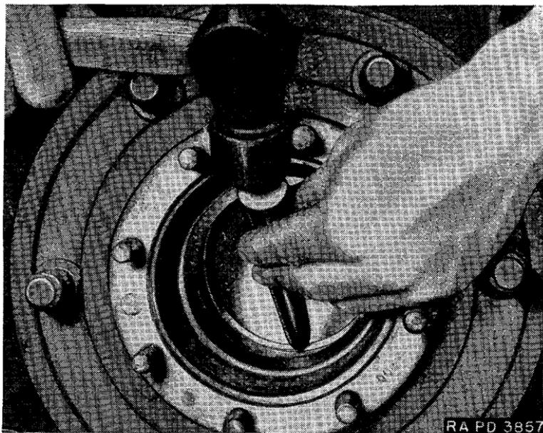
FIGURE 14.—Front axle wheel bearing inner cup removal.
