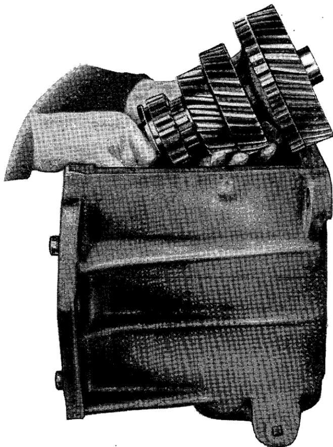
FIGURE 106.—Transmission countershaft removal.
