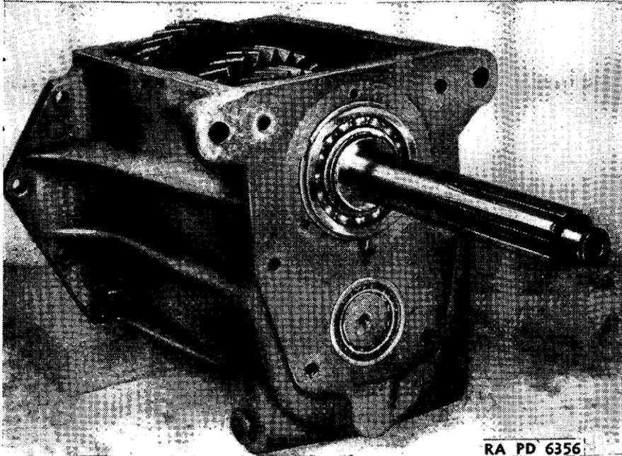
FIGURE 94.—Transmission main drive gear, installed.
