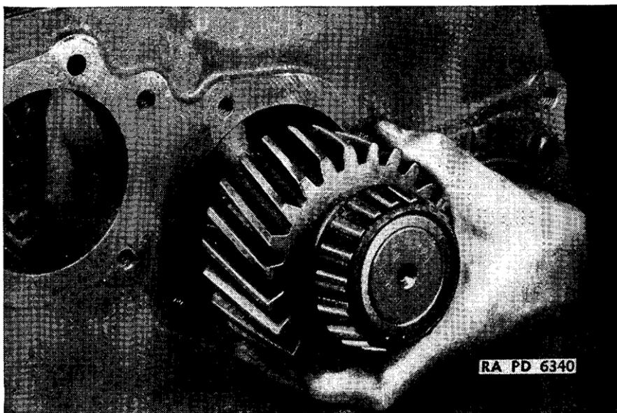
FIGURE 119.—Transfer case intermediate shaft removal.
