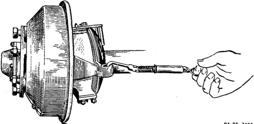
FIGURE 34.—Checking front axle steering knuckle drag.
