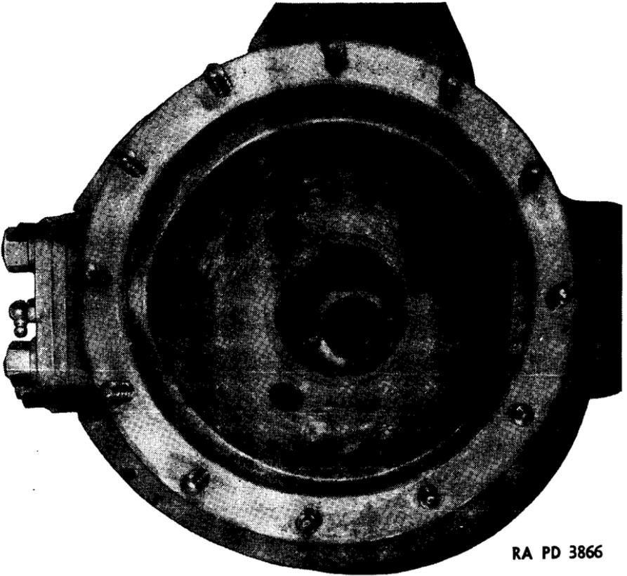
FIGURE 18.—Front axle Rzeppa universal joint housing.
