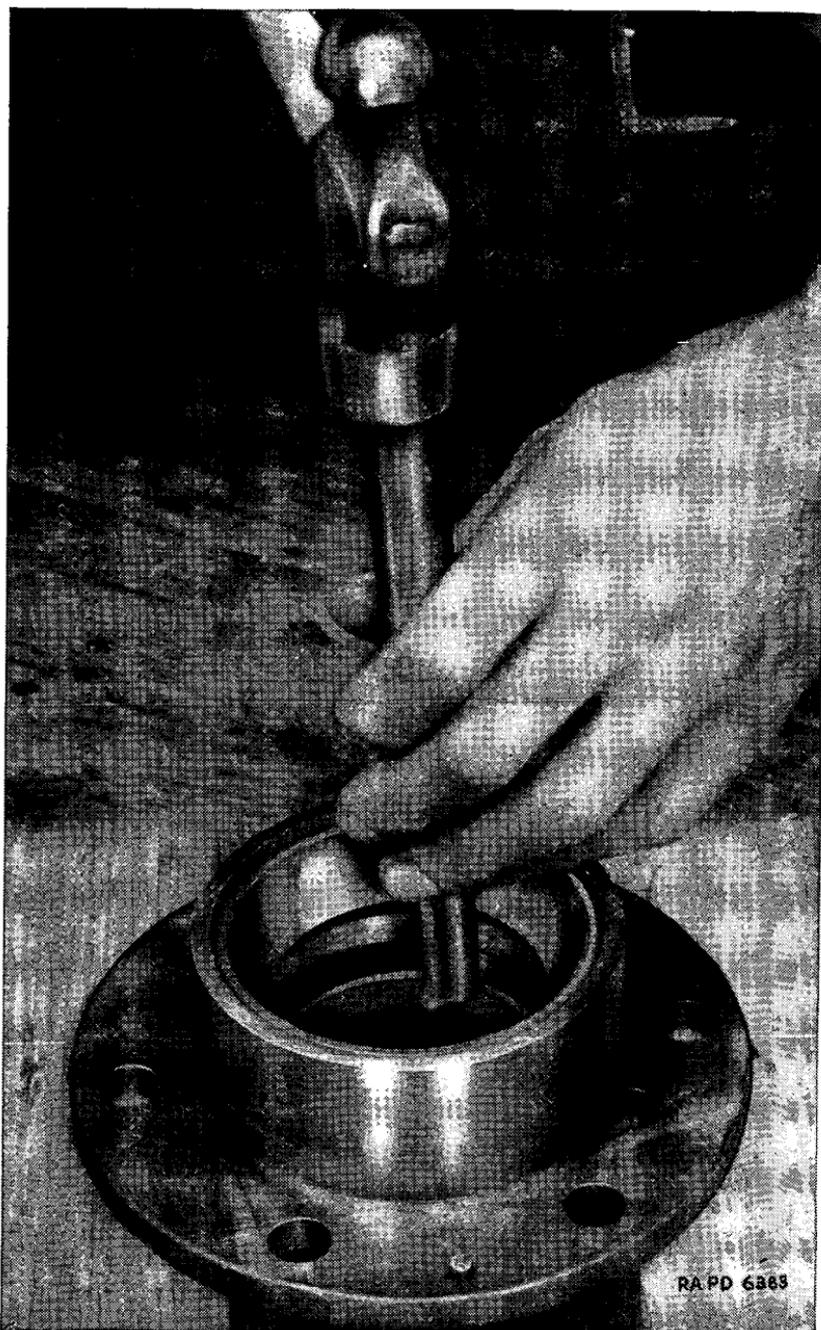
FIGURE 24.—Front axle drive pinion bearing cup removal.
