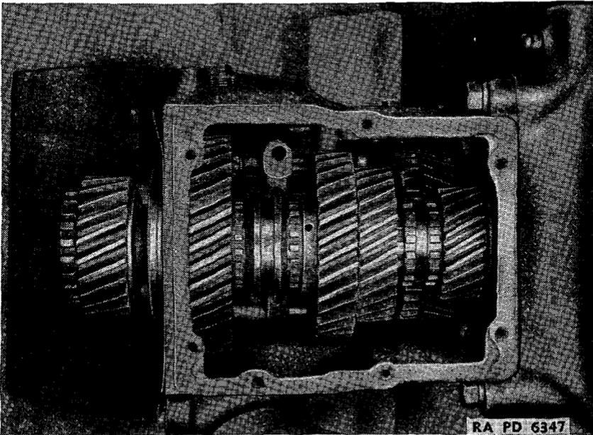
FIGURE 92.—Transmission gears installed.
