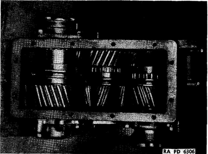
FIGURE 110.—Transfer case gears, installed.
