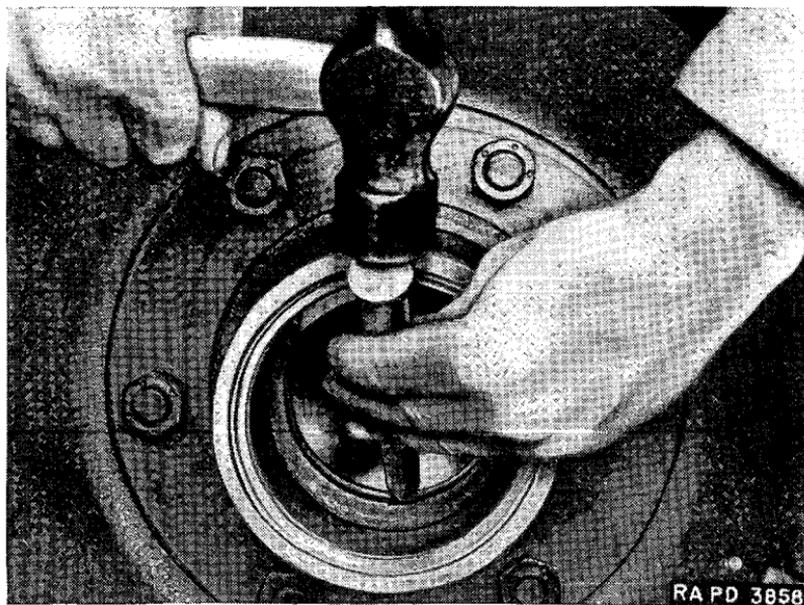
FIGURE 15.—Front axle wheel bearing outer cup removal.
