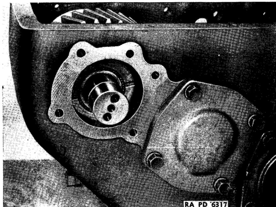
FIGURE 136.—Transfer case front-drive shaft, installed.
