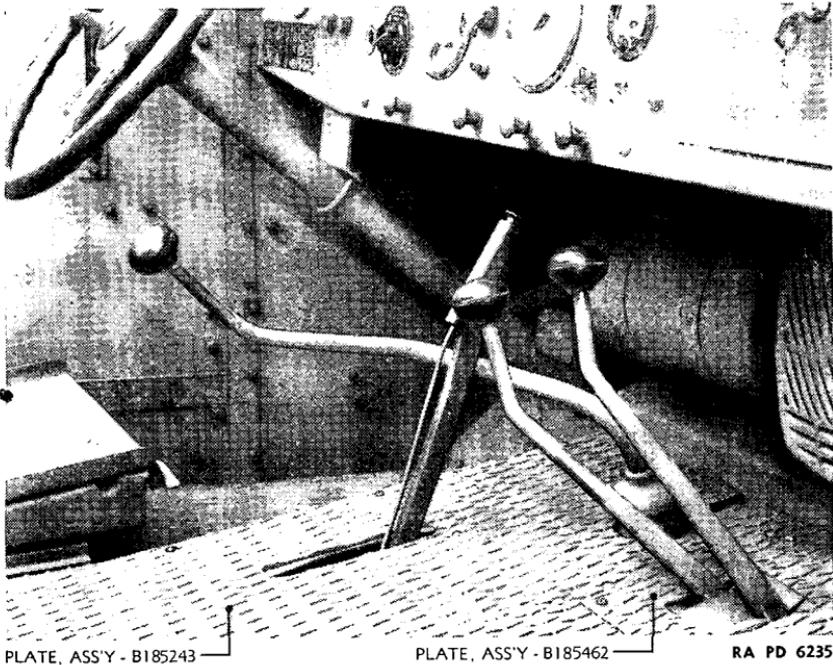
FIGURE 80.—Transmission shift levers and floor plates, installed.
