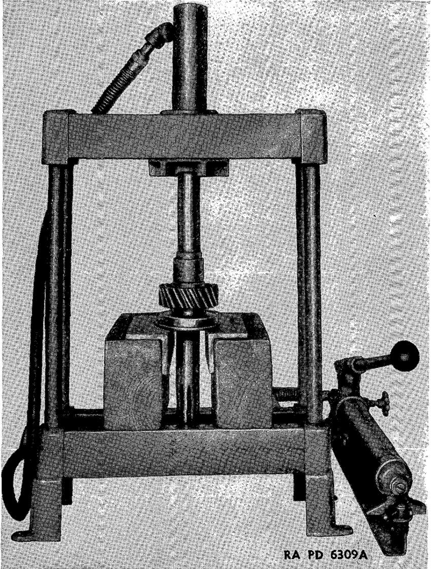
FIGURE 147.—Pressing bearing on transmission main drive gear.
