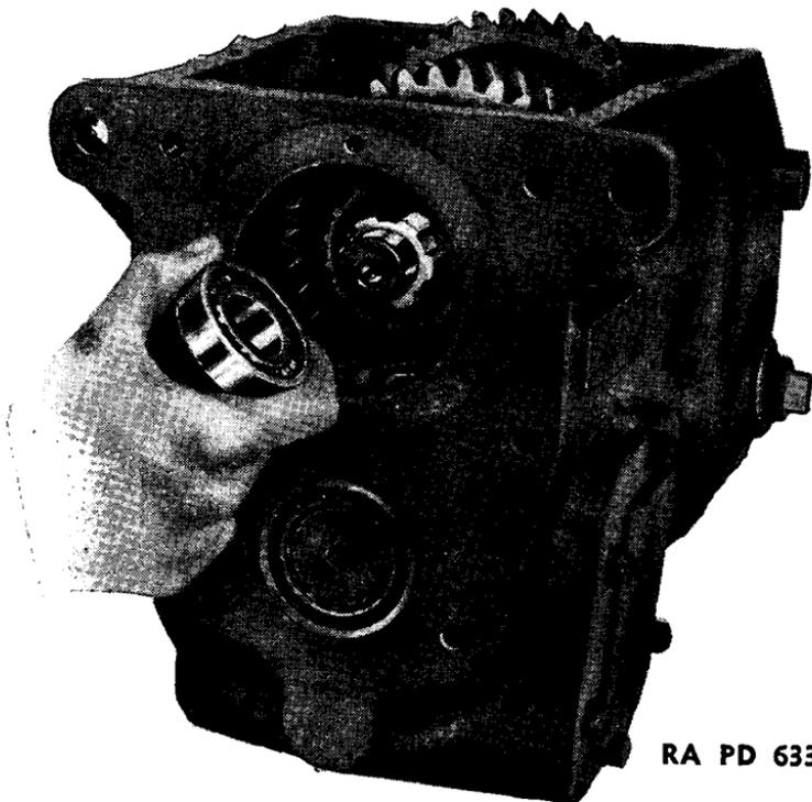
FIGURE 96. -Transmission mainshaft pilot bearing removal.
