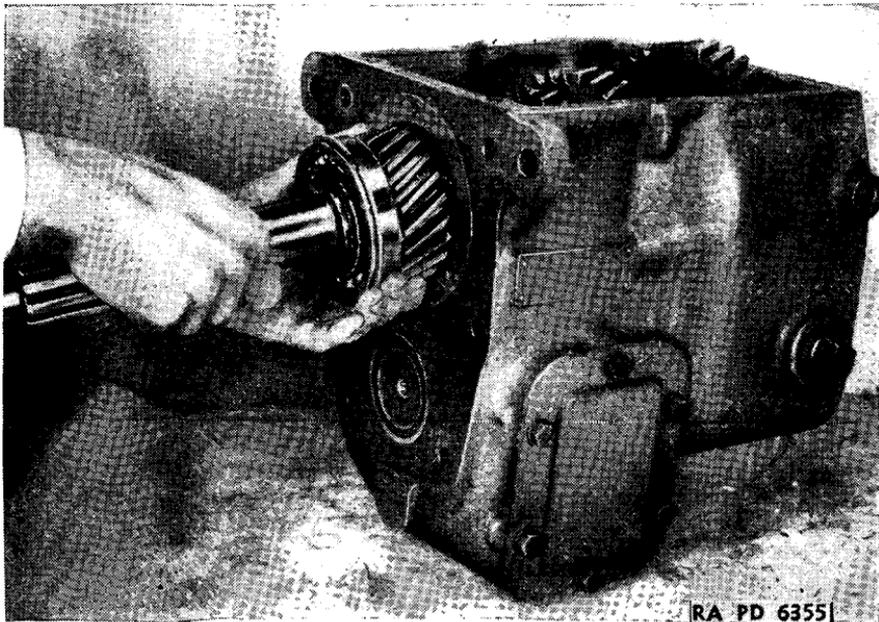
FIGURE 95.—Transmission main drive gear removal.
