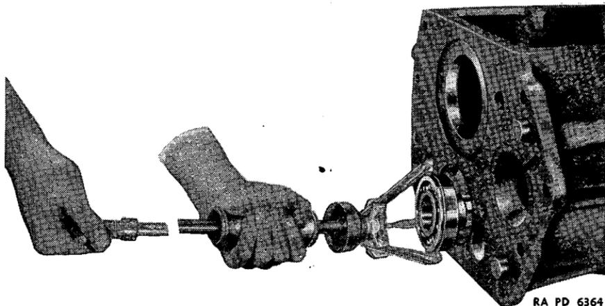
FIGURE 105.—Transmission countershaft rear bearing removal.
