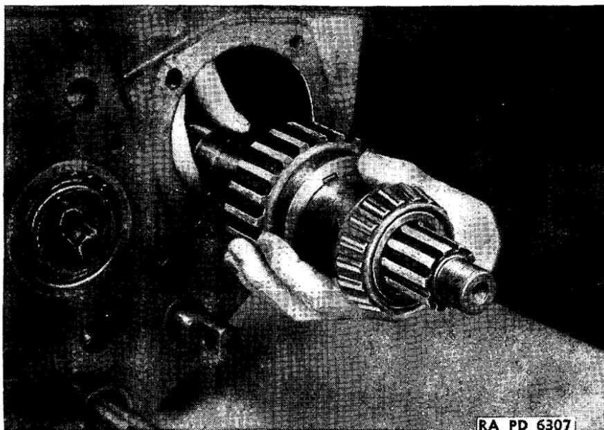
FIGURE 115.—Transfer case front-drive shaft removal.
