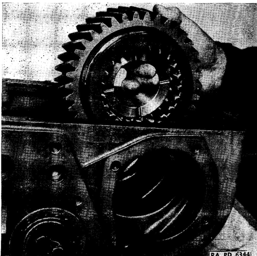
FIGURE 116.—Transfer case front-drive shaft gear removal.
