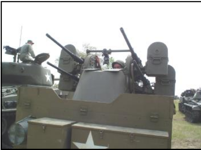
Close-up view of the .50 cal. Quad Mount on the M16 Halftrack
